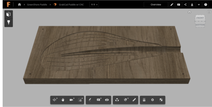
Figure 1: 3d design of a kayak paddle blade for injection molding using water bottles from campus. (Autodesk Fusion 360)
